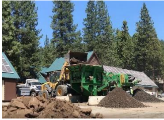
Rock Crushing-Used Native for Backfill (Green Footprint)
